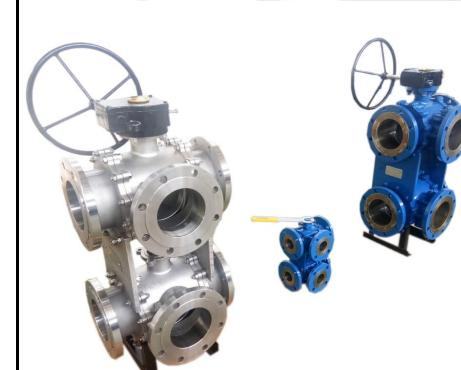
6 Way Ball Valve is designed for Duplex Filters to achieve smooth changeover between the filters. The Valves can be supplied in sizes from 1½ inch to 8 inch full bore. The of Construction Material offered in this range of products is: ASTM A216 Gr WCB Body with CF8/ SS304 trims, ASTM A351 Gr CF8 Body with CF8/ SS304 trims, ASTM A351 Gr CF8M Body with CF8M/ SS316 trims Super Duplex SS Body with Super Duplex SS trims
